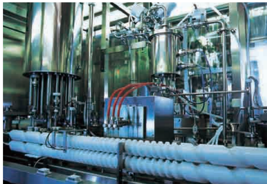
注射筒への溶解液充填 Leuplin powder and solution being filled into the syringe
