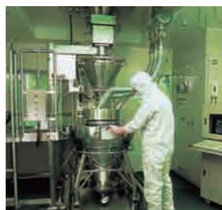
自動秤量機 Weighing machine controlled by a computer
